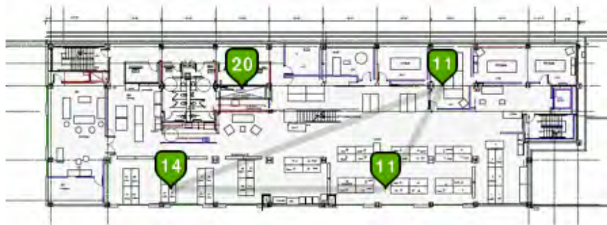
Figure 14 - Good AP Deployment for Accurate Location
