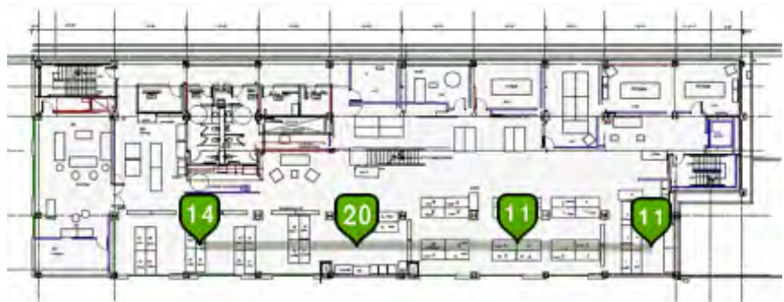
Figure 13 - Poor AP Deployment for Accurate Location
