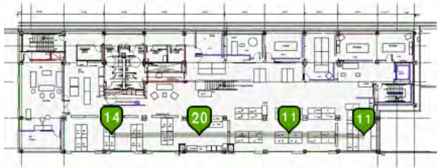
Figure 13 - Poor AP Deployment for Accurate Location
